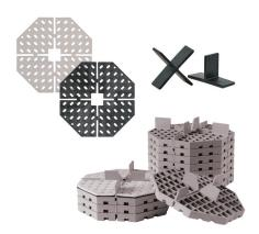
Leveling plates can be used singularly or stacked together to accommodate elevations from 1/16 inch to 5/8 inch (thickness of a support pedestal). Spacer tabs must be used to maintain consistent 1/8 inch joint spacing between pavers.
