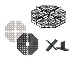
Leveling plates can be used singularly or stacked together to accommodate elevations from 1/16 inch to 5/8 inch (thickness of a support pedestal). Spacer tabs must be used to maintain consistent 1/8 inch joint spacing between pavers.
